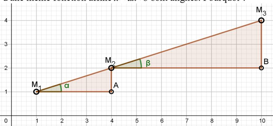
Sur la figure,  $\tan \alpha = \frac{M_2A}{M_1A} = \frac{y_2 - y_1}{x_2 - x_1} = a$  et  $\tan \beta = \frac{M_3B}{M_2B} = \frac{y_3 - y_2}{x_3 - x_2} = a$  ; d'où  $\tan \alpha = \tan \beta$  et donc  $\alpha = \beta$ .
